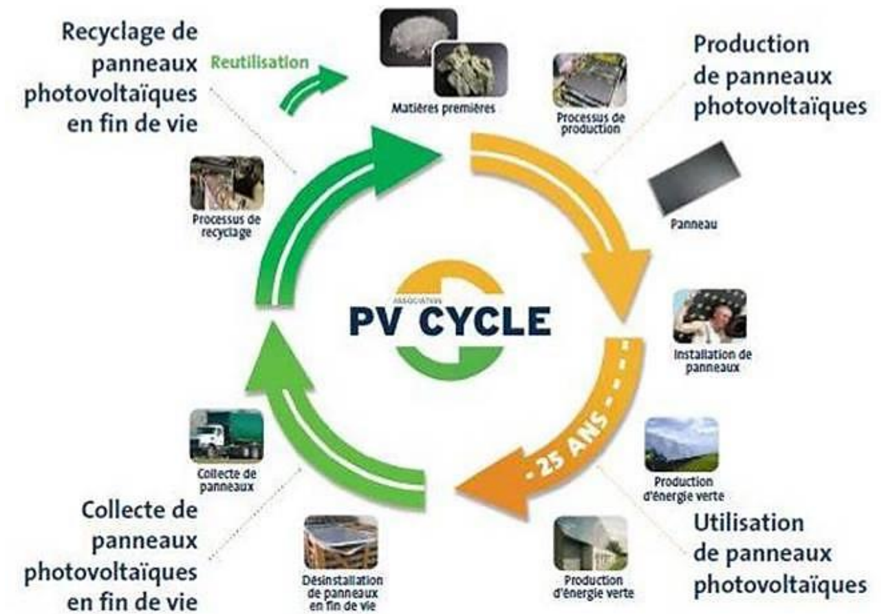
Figure 16. Vie d'une installation photovoltaïque (PV Cycle)
